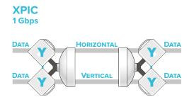
The XPIC system allows to double radio spectrum efficiency. Opposite polarized signals are cancelled out at receiver side. The two channels H and V are independent, reaching a maximum of 500 Mbps each. The best utilization of XPIC is in combination with the Radio Link Aggregation.
